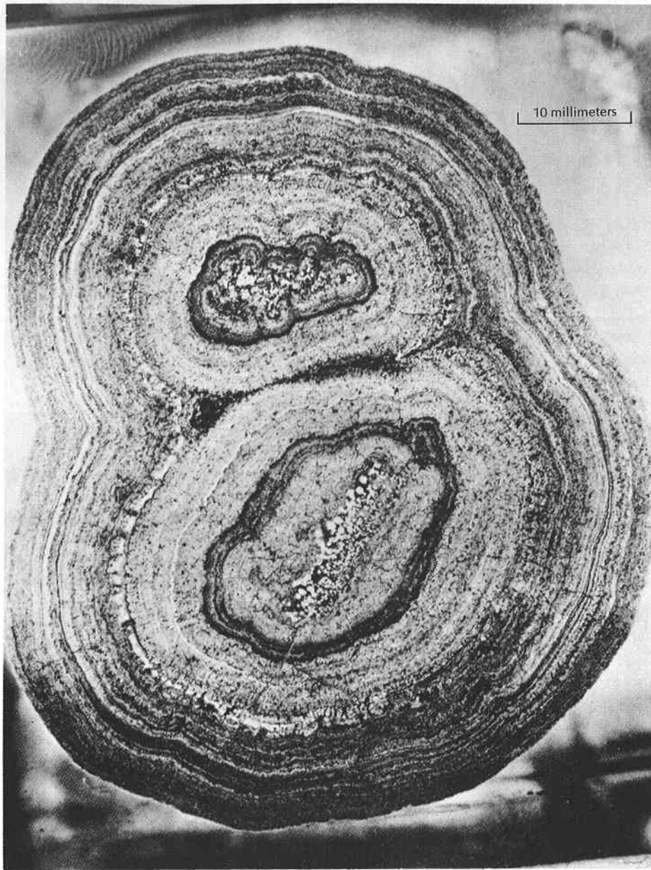
Figure 4-8 Photograph of a cross-sectional cut through a manganese nodule with two growth centers. The altered volcanic material at the centers nucleated the nodule's growth. Crude growth rings representing temporal changes in texture and composition can be seen. This nodule has a radius of 2 centimeters. At a growth rate of 2 mm/ 10^6 yrs, it must have commenced about 10,000,000 years ago.
